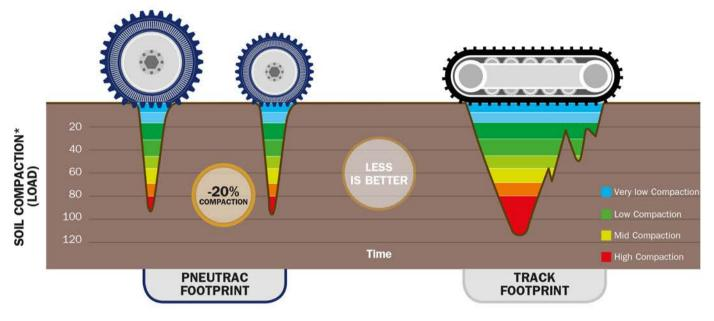
(\*) Load (kg) measured at 10 cm depth by load sensors
